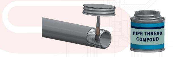
5) Align and support the valve and piping to prevent cross-threading, ensuring the male threaded fitting is properly aligned with the axis of the tapped hole. Maintaining correct pipe support and alignment both during and after assembly helps prevent unnecessary stress on the valve body from the piping.
