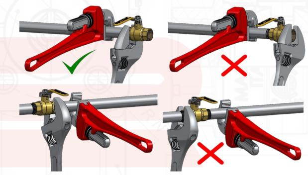
TIP: Brass and bronze alloys are softer than steel, so always use a smooth-jawed wrench on the valve end and rotate the valve onto the pipe. Pipe wrenches should be used only on pipes and fittings.
